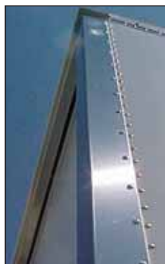
◀ Stainless steel frame – standard on any body with tandem axle reinforcement package, optional on other bodies.
